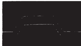
Fig. 18 – Typical square wave response at V_{DD} = V_C = +10 V, V_{SS} = Gnd .
